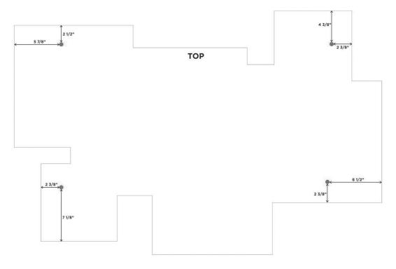
mounting pattern with 4 anchoring holes marked on clear acylic backer only
